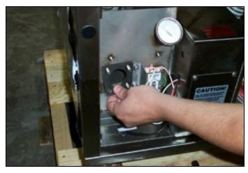
Removing the heater gasket
